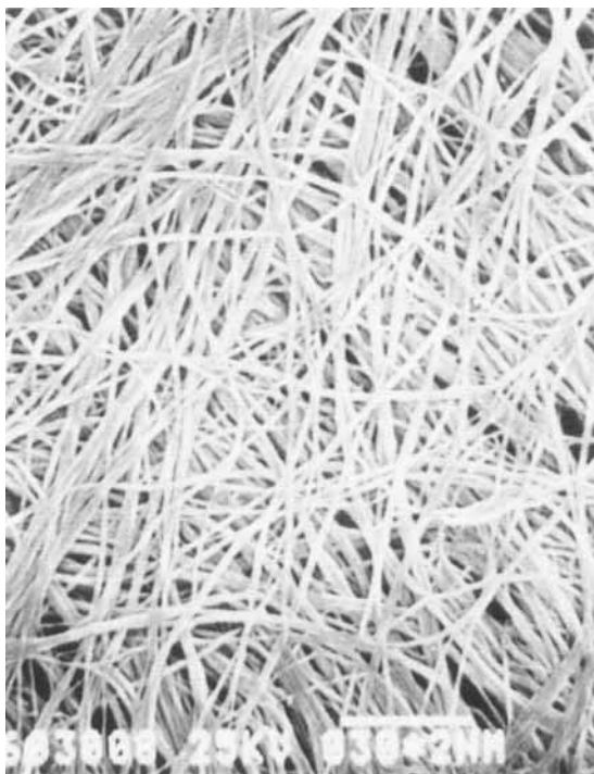
FIG. 3. Scanning electron micrograph of a polyacetylene film prepared in a quiescent nematic phase of the catalyst solution.
